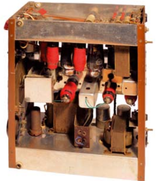
The 88-10 AM receiver amplifier dating from the very early 1950s and featuring the standard Mullard range of octal valves available at the time. This set has an abundance of EBC33s, three of which are strapped as triodes. As there appears to be no technical advantage it has to be assumed that these valves were obtained at such a low price that it worked out cheaper to produce like this. Provision is made for gram and for feeding into further amplifiers. The output pair are EL33s. Note the use of a moving coil meter to indicate signal strength. The set still has its previous owner's badge declaring it Equipment Number 4, Surrey County Council. The cabinet is made of solid oak. The similarly designed later series were manufactured from oak-faced ply.
