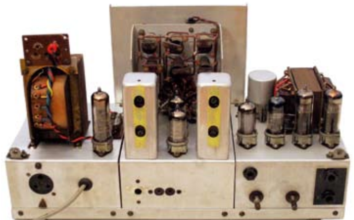
Centre right and right: The chassis of the SB4 showing the neat and modular layout of the set, a feature that would be retained on many of the later designs. The valve line up is typical of a period superhet with the B8A range of valves being employed these being EZ40, ECH42, EF41, EBC41, ECC40 and two EL41s. A 4 Watt output is claimed from the set. A gram socket is located on the rear along with the bass and treble controls.
