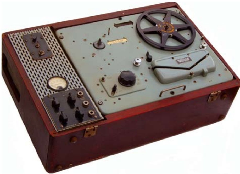
Left: When Vortexion entered the semi professional recording market they had already gained some experience with the design and manufacture of amplifiers for magnetic tape and direct to disc recording. A rare example of an early WVA tape recorder outfit pictured here on the left, first appeared in early 1953 and features the Series 2 Wearite deck, although it was also briefly offered with the Truvox deck as an option. Vortexion continued their range of recorders based on this design until the demise of the Wearite deck in 1968. A new model that briefly appeared featuring the Ferrograph Series 7 deck, and known as the CBL7T can be seen above
