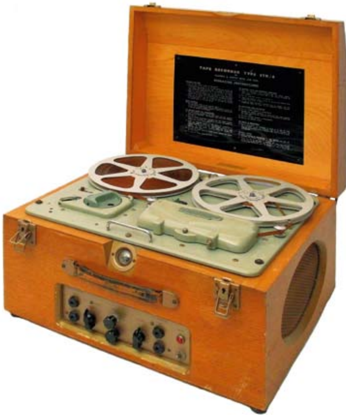
Above: The STR 4 tape recorder from 1959 featuring the Ferrograph Wearite Series 4 deck was a good performer in terms of facilities and overall quality. This equipment was also made available to the general public.
