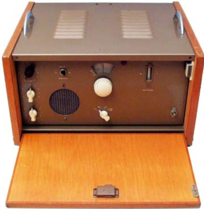
The later 88-20 AM/FM receiver amplifier. This example dates from the mid 1960s and followed the well established cabinet tradition with the drop down lockable flap. This example features EL84s in a parallel push pull arrangement and a semiconductor based FM tuner. Various versions of the 88 series were produced over the years, the second generation AM only equipment for example, and originally featured B8A valves throughout with parallel push pull EL41s and a neon tuning indicator. EM34s or EM84s will also be found as the tuning indicator in some models. The earliest of the 88 series FM models featured a valve based "bought in" tuner utilising an ECC85 which was prone to periodic drifting.
