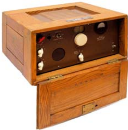
The 88-10 AM receiver amplifier dating from the very early 1950s and featuring the standard Mullard range of octal valves available at the time. This set has an abundance of EBC33s, three of which are strapped as triodes. As there appears to be no technical advantage it has to be assumed that these valves were obtained at such a low price that it worked out cheaper to produce like this. Provision is made for gram and for feeding into further amplifiers. The output pair are EL33s. Note the use of a moving coil meter to indicate signal strength. The set still has its previous owner's badge declaring it Equipment Number 4, Surrey County Council. The cabinet is made of solid oak. The similarly designed later series were manufactured from oak-faced ply.
